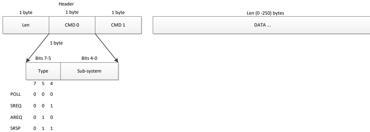
Figure 5: Standard MT Frame Format
